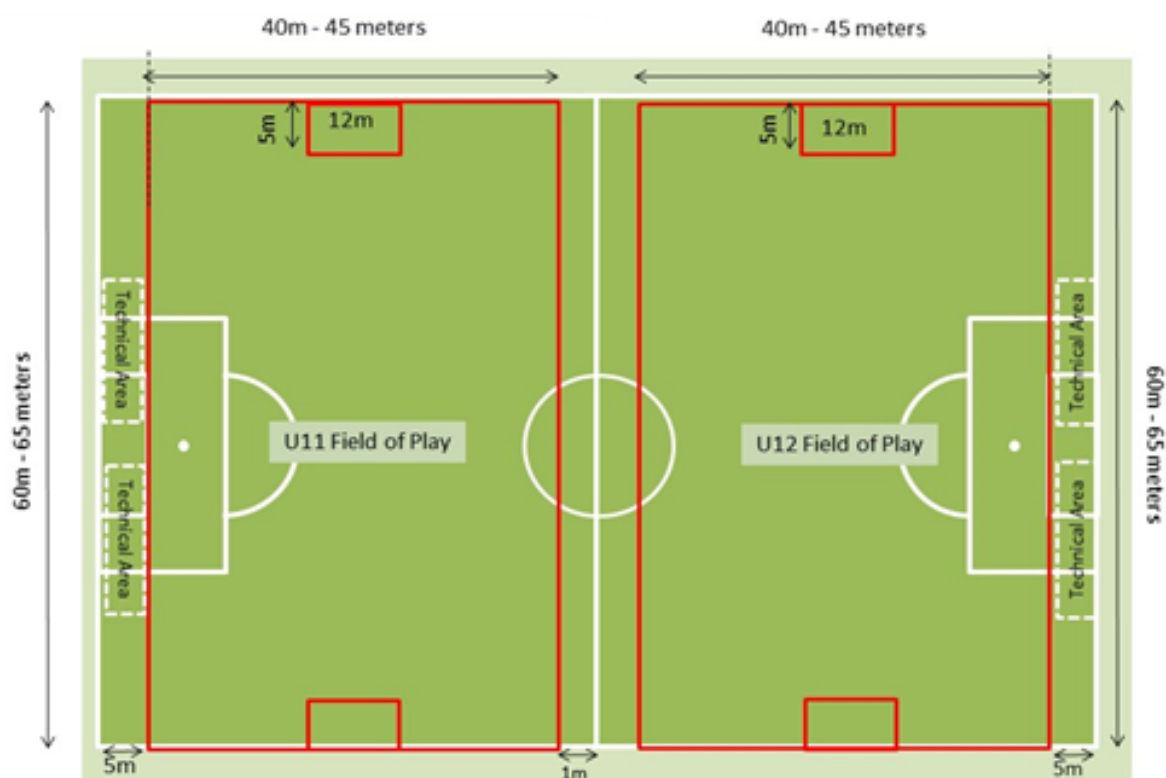
Diagram 4 - U11 and U12 Preferred Field Orientation OPTION 1
